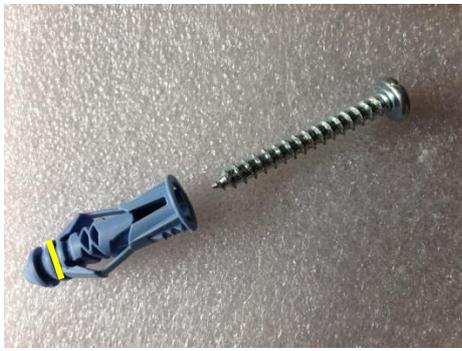
Wall fitting. Drill a hole of diameter shown by yellow line. Tap plastic component until it is embedded in plaster wall. Metal screw through the panel is driven into end.
