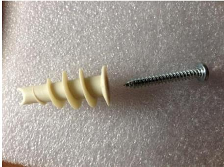
Ceiling fitting. Using a Philips screwdriver, make a hole in plaster ceiling and screw in plastic component (cutting its own path). Metal screw through panel is then driven into end
